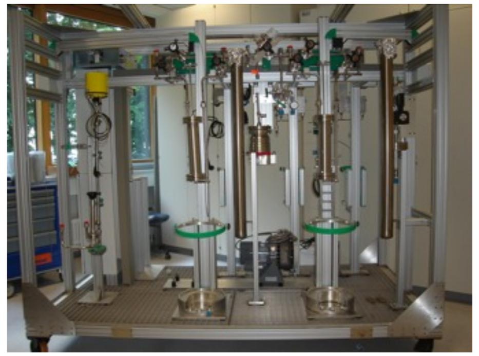
Mobile Radon Extraction unit (MoREx) @ MPIK to test efficiency of various charcoals for Rn removal from Xe
